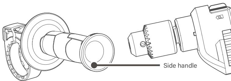
Please always use the side handle to ensure safe operation. Install the side handle onto the installation tube of the tool.
